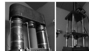
Remotely operated precision 180t and 10t presses.
